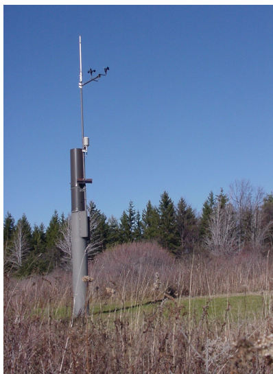
Climate station transmits real-time data for precipitation, air temperature, barometric pressure, relative humidity, wind speed, and wind direction.
