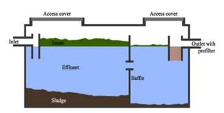
Wastewater leaving the tank flows through an **OUTLET FILTER** to a **DISTRIBUTION BOX**. This box allows the effluent to flow evenly into several **PERFORATED PIPES** that disperse effluent into the soil. The Soil area is called an **ABSORPTION FIELD** (also commonly called a leach field).
